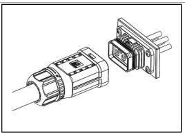
2. Separate the female cable end connector and male panel mount connector.
