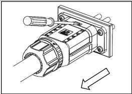
1.Press the part of unlocking position through the screwdriver, synchronously hold and pull out the female cable end connector to separate the female and male connectors.
