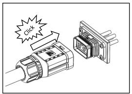
5.Insert the female cable end connector into the male panle mount connector and hearing the "Click" sound.
