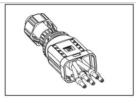
1. The stripped wires need to be riveted to the insulated terminals, and after then, thread them into the wire-locking nut and connector mainbody in turn.
