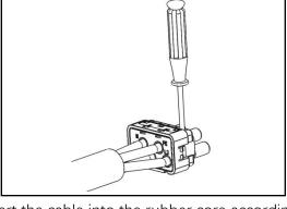
2.Insert the cable into the rubber core according to the wire sequence, make sure the insulated terminal flush with the rubber core surface, and the torque of the crimping screwdriver is 2.0  $\pm$  0.1N. m
