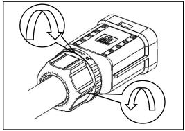
3.Hold the unlocking buckle and rotate it in the marked direction, and rotate the nut in the opposite direction with another hand.
