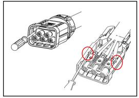
4.Use a screwdriver to peel off the part cycled in red color as shown on both sides to complete the unlock.
