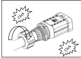
4. Tighten the nut with an open\_x0002\_ended wrench and complete the installation with a "click, click" sound.
