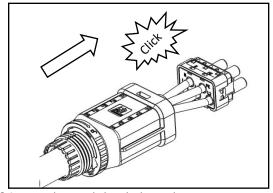
3.Insert the mainbody into the connector rubber core and hearing the "click" sound.
